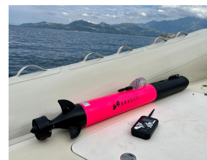
YUCO-eDNA and SEACOMM UHF hand-held radio command unit. picture credits, MARBEC Institute, Montpellier.
