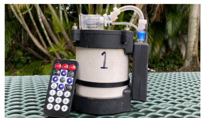
The sub-surface automated environmental DNA (eDNA) sampler (SAsE) submersible to 55 meters of depth.
