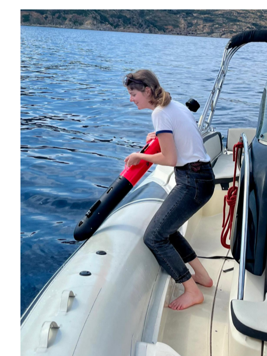
[left-side picture] Operator performing the arming sequence of the YUCO-eDNA prior to launching. Following LED indicators in the mast
