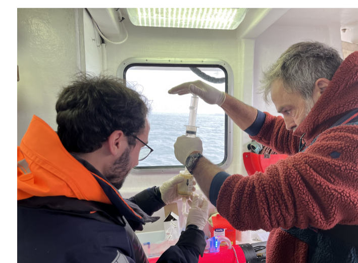
Filling the filter with CL1 buffer solution from VIGILife. picture credits - IUEM - UBO Brest
