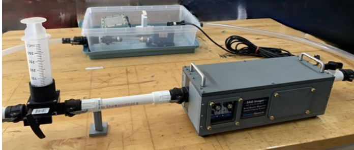
Desktop system for single-pass imaging of previously collected samples
